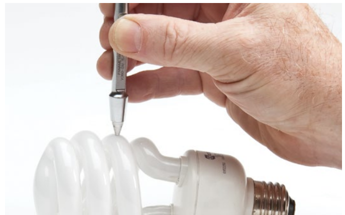
The High Resolution software option enables thickness measurements of up to 0.001 mm (0.0001 in.) resolution.
