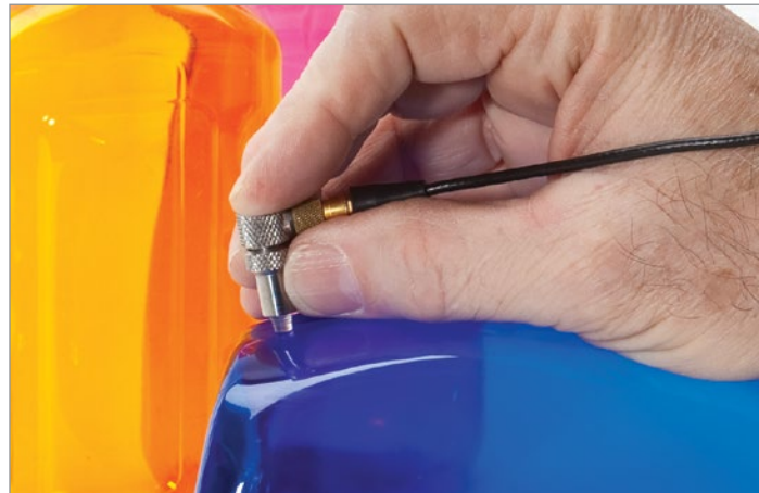
Measure thin plastic material using a 20 MHz delay line transducer.
