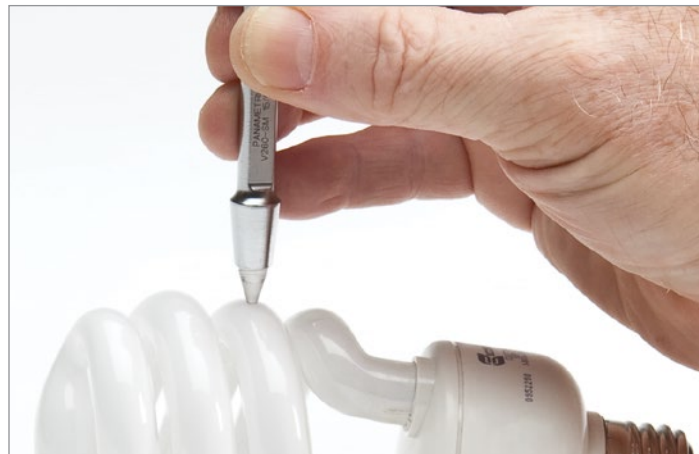
Measure thin glass with a V260-SM Sonopen® transducer.
