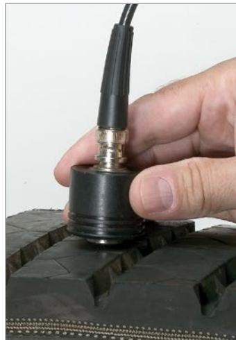
Measure depth to steel ply / cords in rubber conveyor belts or tires.
