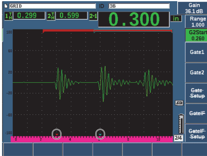
Figure 11-43 Echo measurement error
