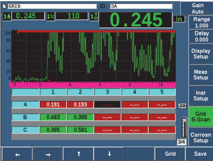
Figure 11-37 Corrosion Module grid view
