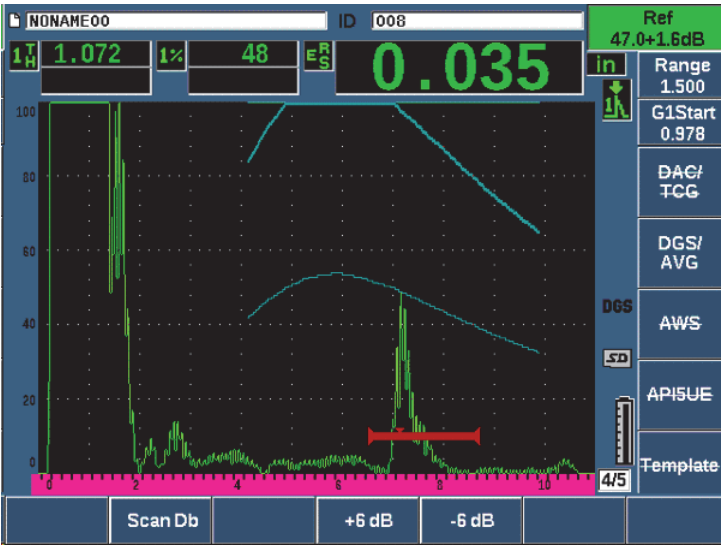
Figure 11-17 Gain curve adjusted DGS
