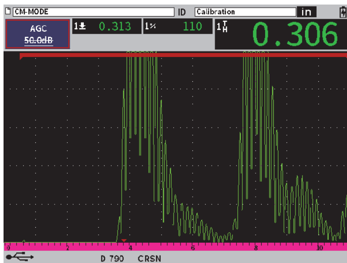
Figure 11-37 Incorrectly triggered measurement
