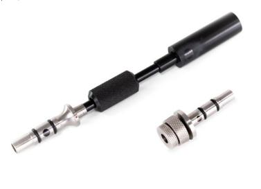
Connector: 4-pin universal Fischer connectorFrequency range: 200 kHz–3 MHz
