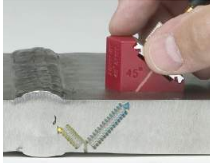
Miniature angle beam transducers and wedges are used primarily for testing weld integrity. Their design enables them to be easily scanned back and forth and provides a short approach distance.
