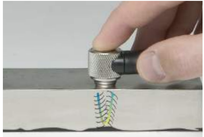
Two angled elements create a V-shaped sound path in the test material. This pseudo-focus enhances resolution in the focal zone.
